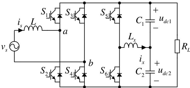
Fig. 1. The topology of the single-phase power converter with DC-split-capacitor power decoupling circuit.
