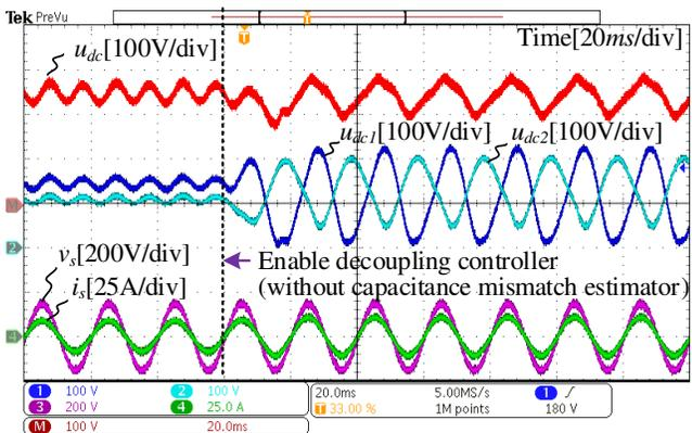
Fig. 8. Experimental results of the decoupling controller start-up in Case II (without capacitance mismatch estimator).
