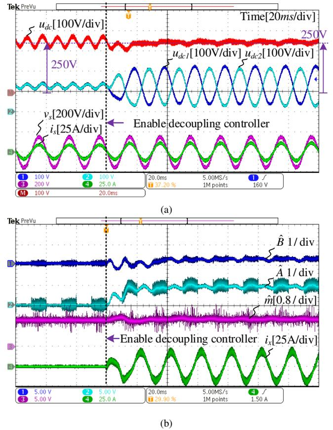
Fig. 6. Experimental results of the decoupling controller start-up in Case I (with capacitance mismatch estimator). (a) Waveforms of capacitor voltages  $u_{dc1}$  and  $u_{dc2}$ , DC-link voltage  $u_{dc}$ , the input AC voltage  $v_s$  and current  $i_s$ ; (b) Waveforms of the estimated values of  $A$ ,  $B$ , and  $m$ , the inductor current  $i_x$ .
