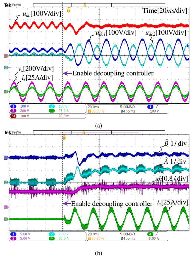
Fig. 9. Experimental results of the decoupling controller start-up in case II (with capacitance mismatch estimator). (a) Waveforms of capacitor voltages  $u_{dc1}$  and  $u_{dc2}$ , DC-link voltage  $u_{dc}$ , the input voltage  $v_s$  and current  $i_s$ ; (b) Waveforms of the estimated values of  $A$ ,  $B$ , and  $m$ , the inductor current  $i_x$ .
