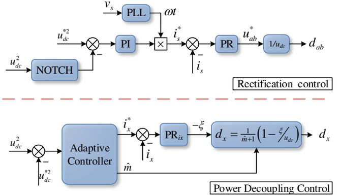
Fig. 2. Proposed control diagram for single-phase power converter with DC-split-capacitor power decoupling circuit.
