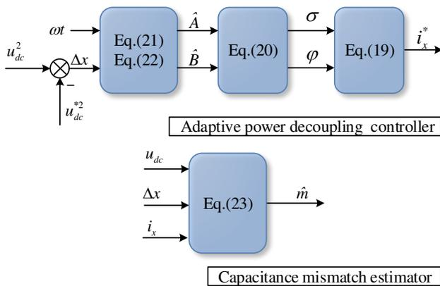
Fig. 3. The diagram of the proposed power decoupling controller.
