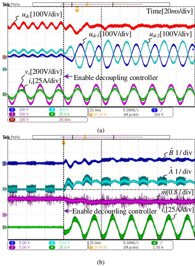
Fig. 11. Experimental results of the decoupling controller start-up in Case III (with capacitance mismatch estimator). (a) Waveforms of capacitor voltages  $u_{dc1}$  and  $u_{dc2}$ , DC-link voltage  $u_{dc}$ , the input voltage  $v_s$  and current  $i_s$ ; (b) Waveforms of the estimated values of  $A$ ,  $B$ , and  $m$ , the inductor current  $i_x$ .
