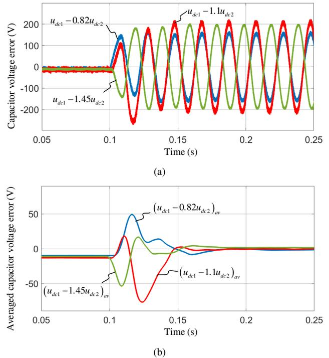
Fig. 12. Waveforms of calculated variables. (a) Waveforms of the capacitor voltage error  $u_{\Delta}$ ; (b) Waveforms of the capacitor averaged voltage error  $u_{\Delta av}$ .
